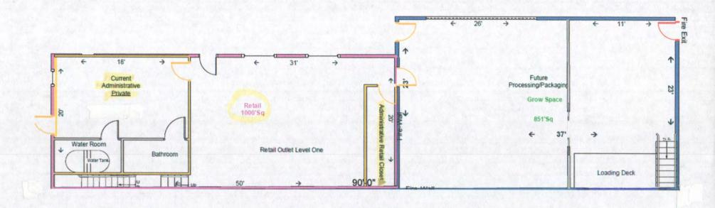
Drawing here has a proposed change in the original drawing to reduce the retail store to a 1000sq' retail outlet on the first floor only, this would reduce the retail from 2000sq' with a consumption venue to 1000sq' with the consumption venue removed.
