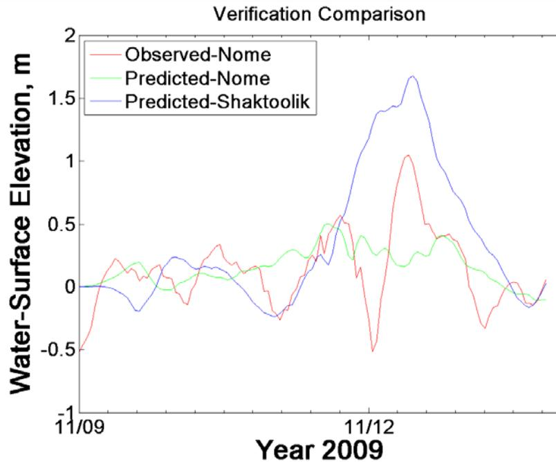
Figure 3-8. Comparison of observed water levels at Nome, AK with predicted at Nome and Shaktoolik during November 2009.
