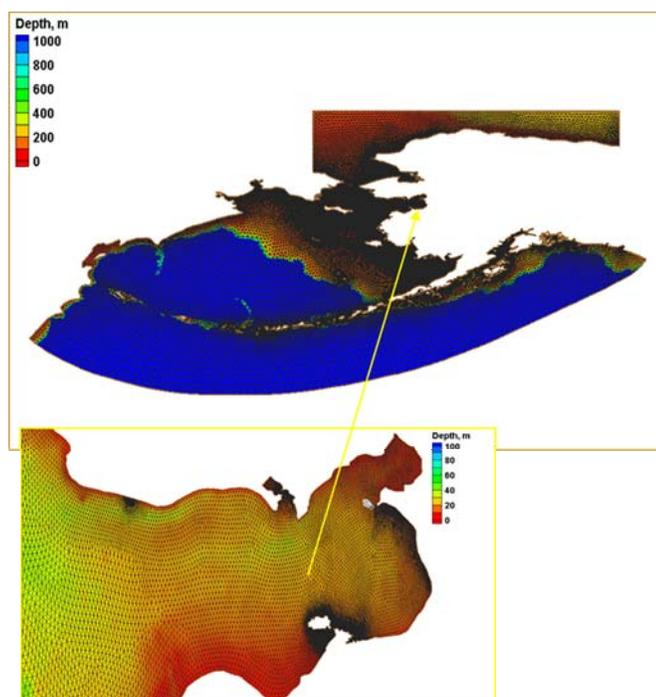
**Figure 11 – ADCIRC Grid for Alaska Coast and Refined for Norton Sound**
