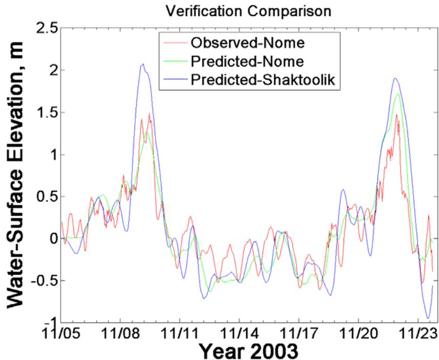
Figure 3-6. Comparison of observed and modeled water levels at Nome; November 2003.
