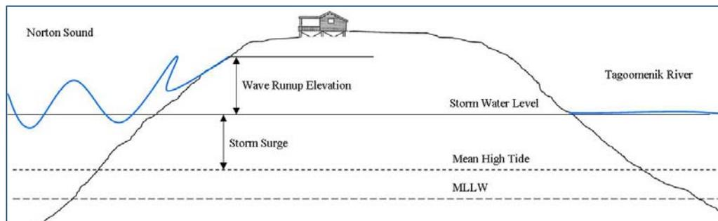
**Figure 8 – Schematic Illustration of Wave Effects**
