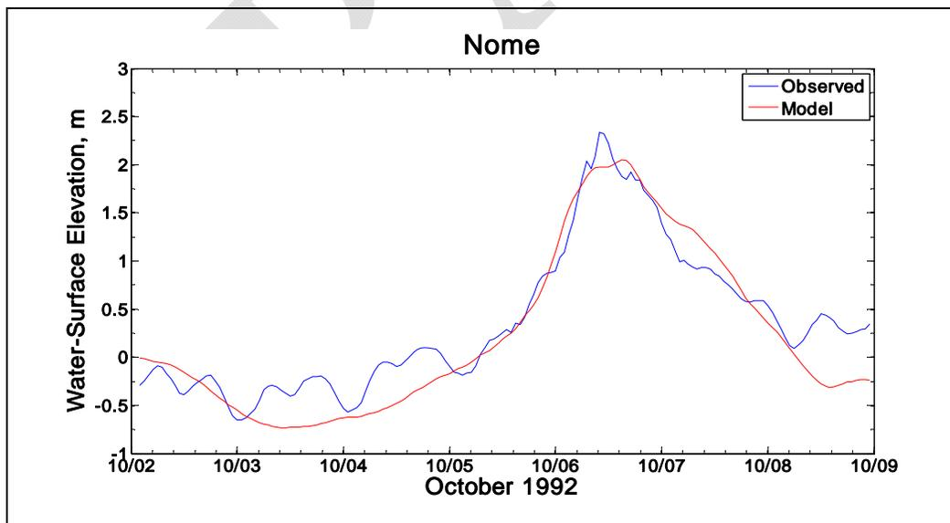
Figure 3-5. Comparison of observed and modeled water levels at Nome, AK; October 1992.
