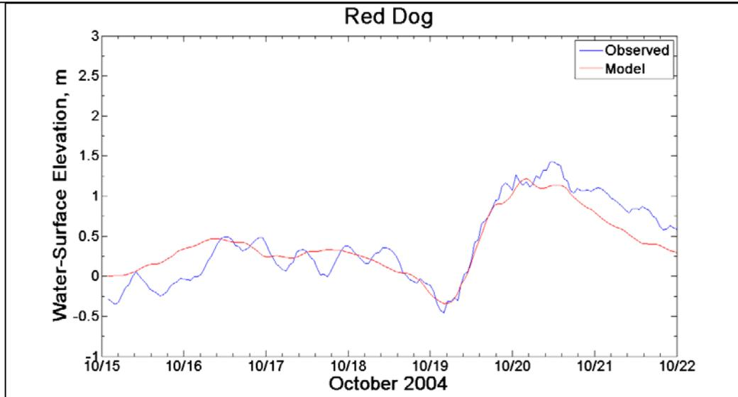
Figure 3-4. Comparison of observed and modeled water levels at Red Dog,; October 2004.
