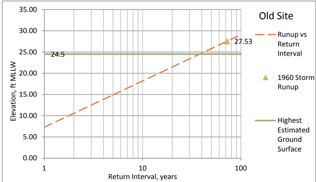
**Figure 14 - Old Site Profile Comparison of Runup to Storm Damage Report**
