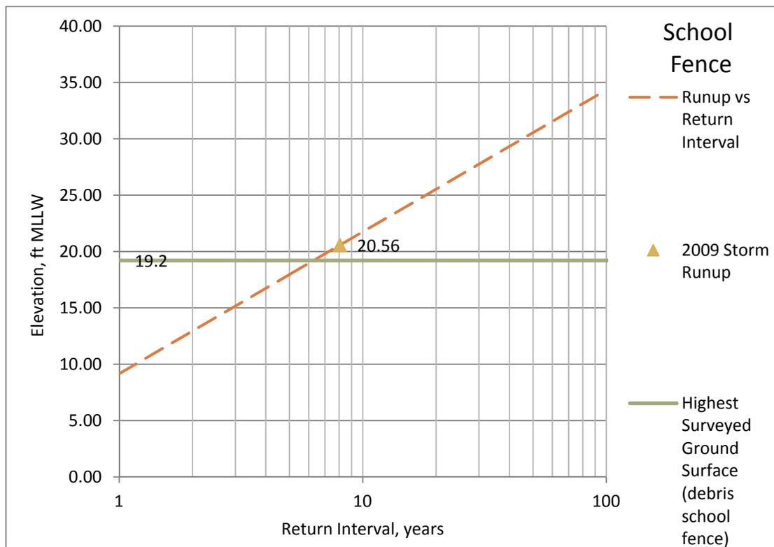
**Figure 16 – School Building Profile Comparison of Runup to Storm Damage Report**
