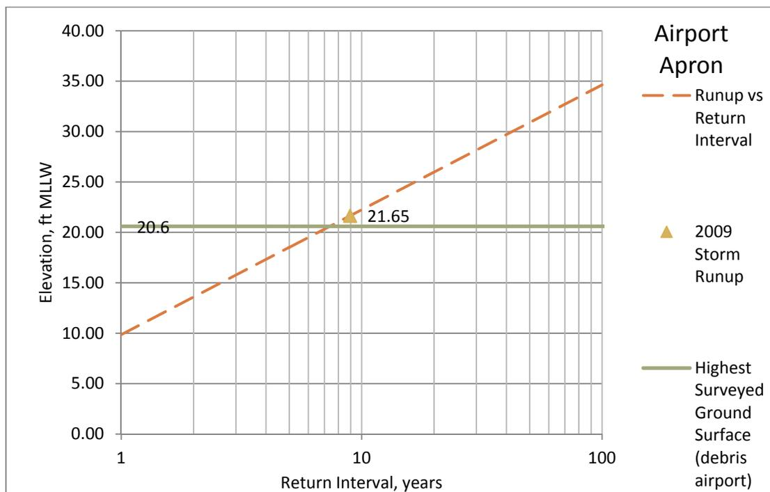
**Figure 17 – Airport Apron Profile Comparison of Runup to Storm Damage Report**
