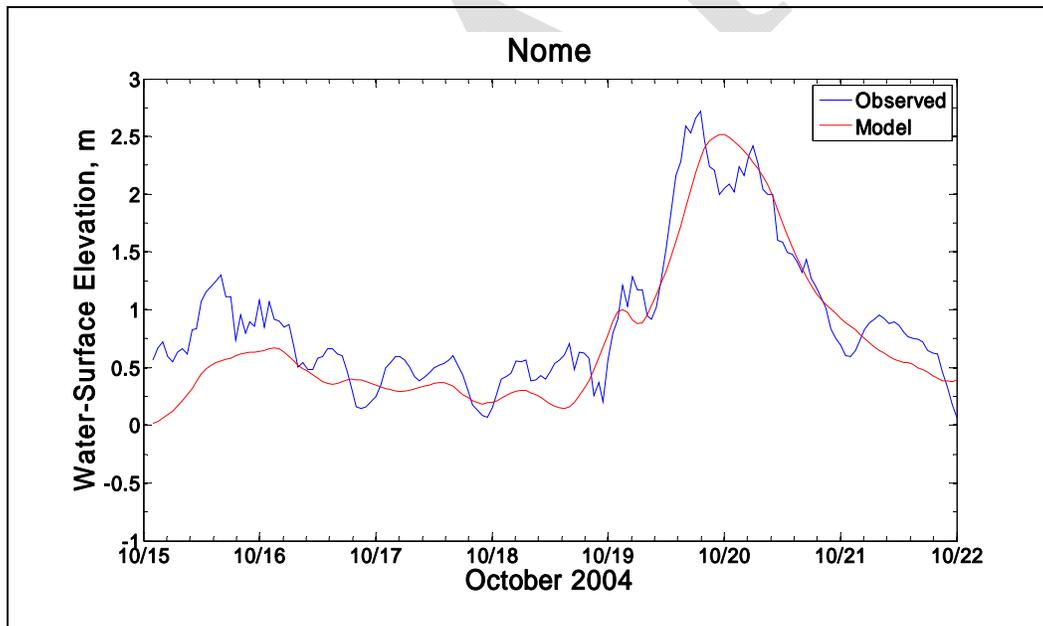
Figure 3-3. Comparison of observed and modeled water levels at Nome; October 2004.
