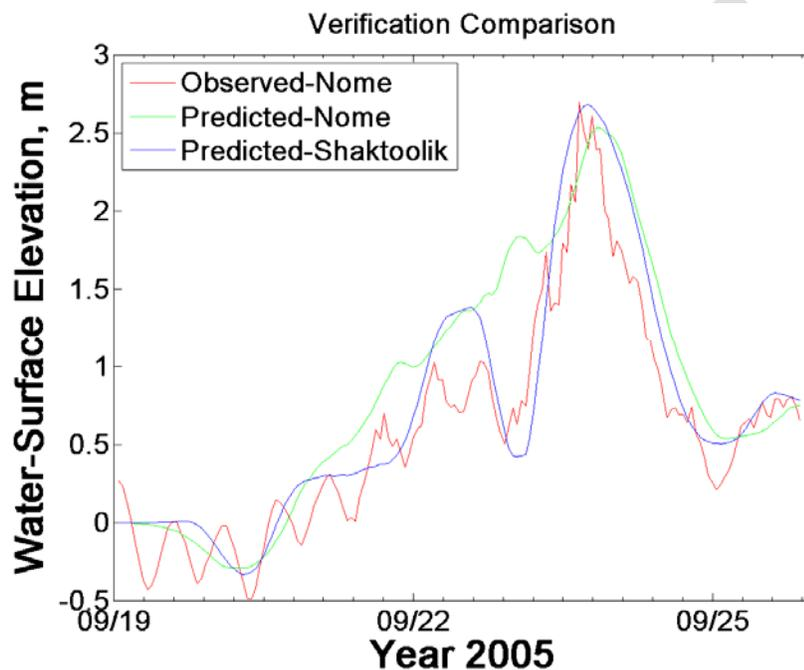
Figure 3-7. Comparison of observed water levels at Nome, AK with predicted at Nome and Shaktoolik during September 2005.
