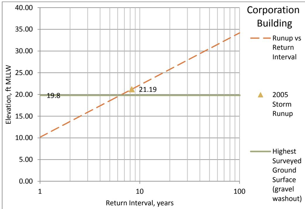
**Figure 15 – Corporation Building Profile Comparison of Runup to Storm Damage Report**
