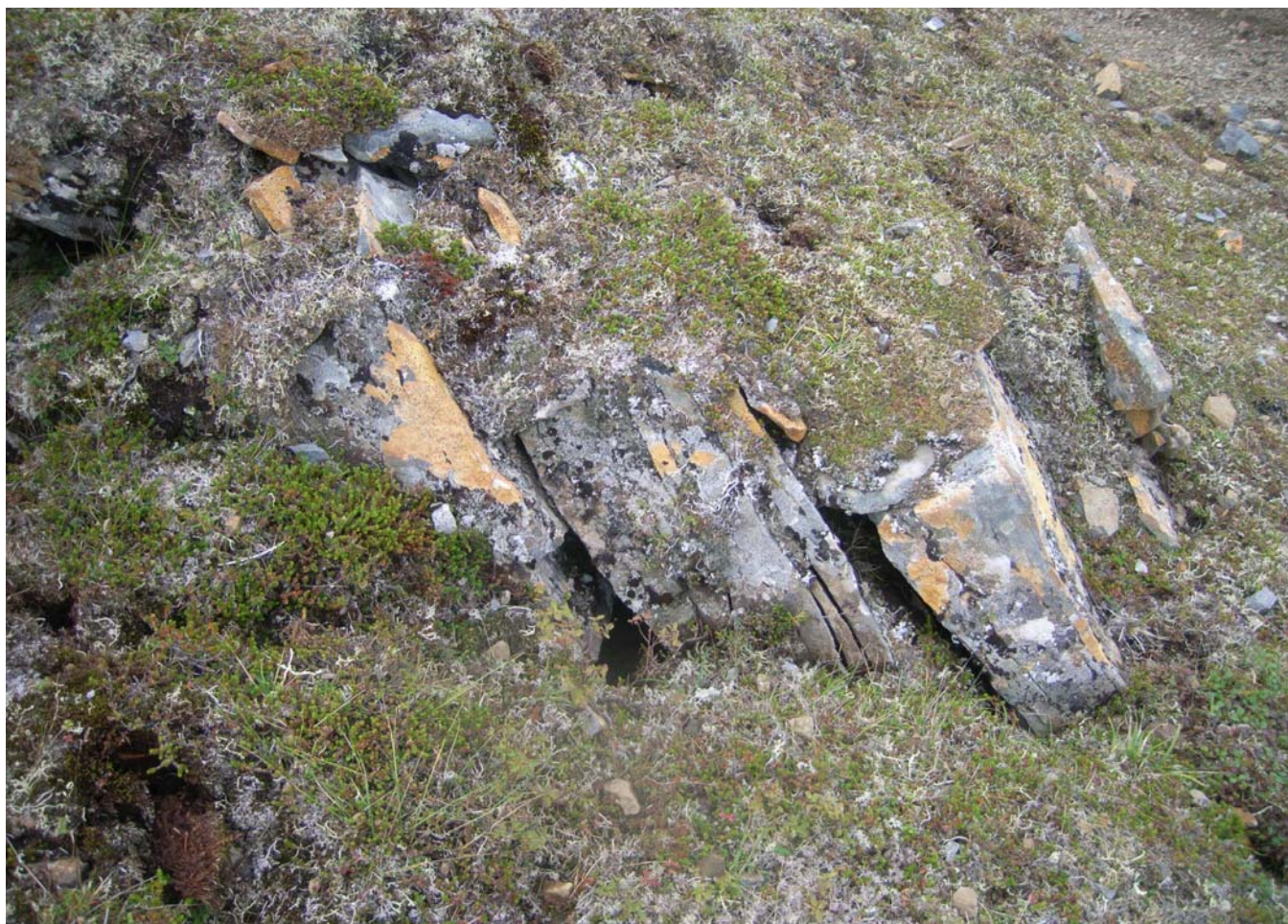
Bedrock with 2-4 inch spaced joint sets
