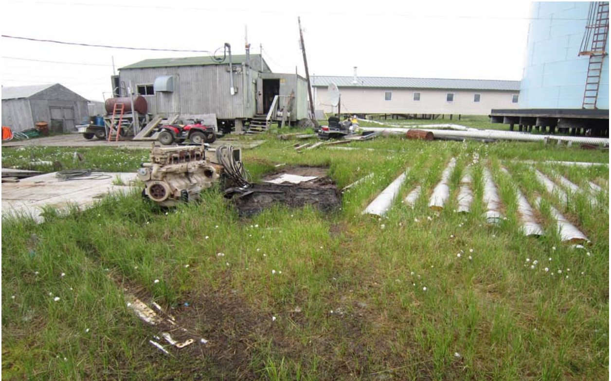
Photo 30: Oil stained soil near genset motor.
