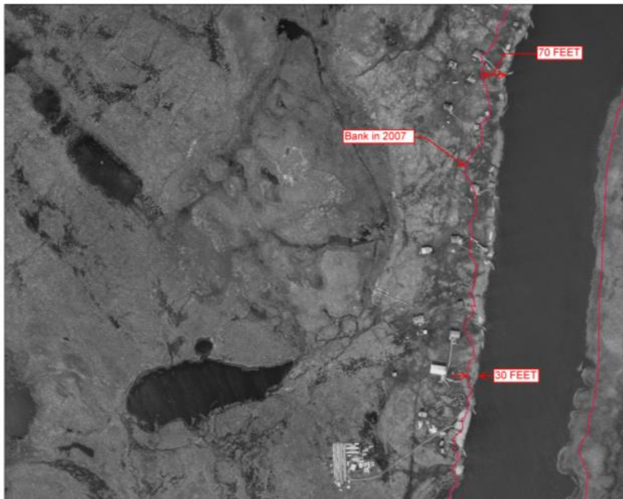
Figure 4: Bank retreat from erosion on Pitmiktakik River, from 1971 (photo) to 2007 (red line).
