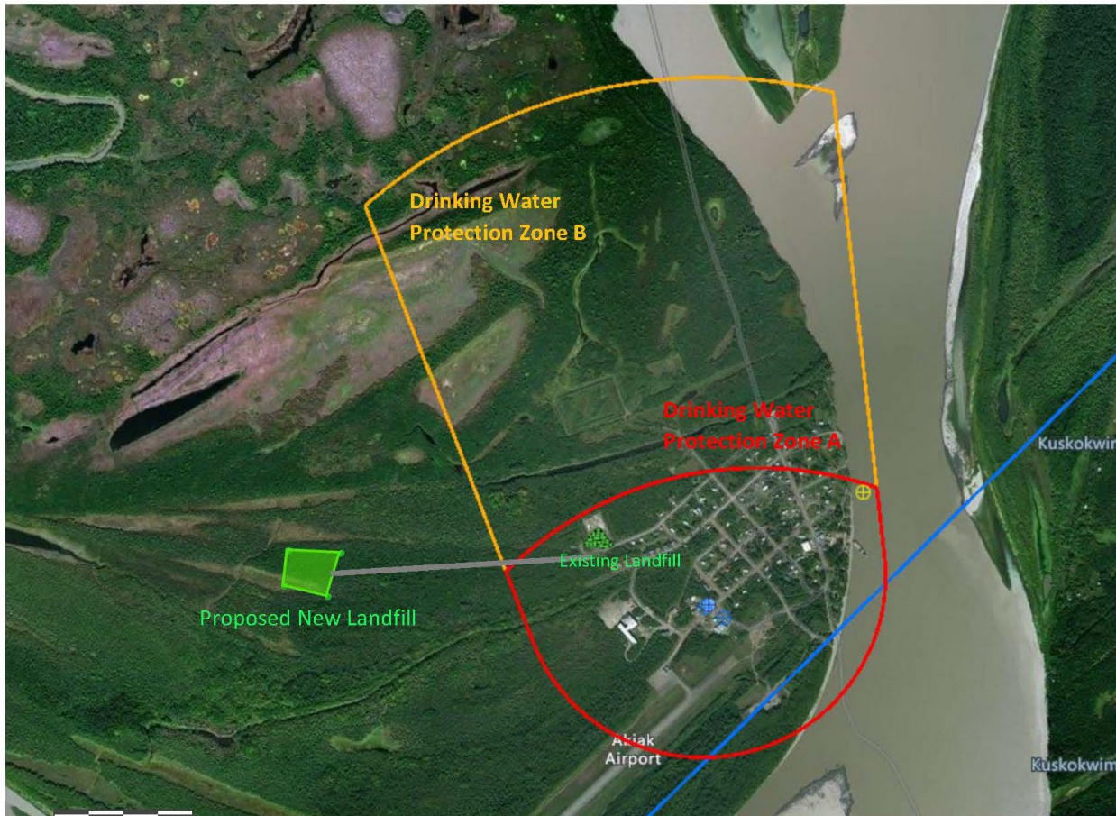
Location of the existing Akiak Landfill in Drinking Water Protection Zone A and the Proposed New Landfill which is planned to be sited outside of Drinking Water Protection Zones A and B
