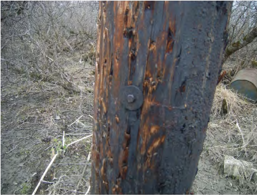
Photo 1: High water marker indicating the level of the flood of record designated ARHW in this survey.
