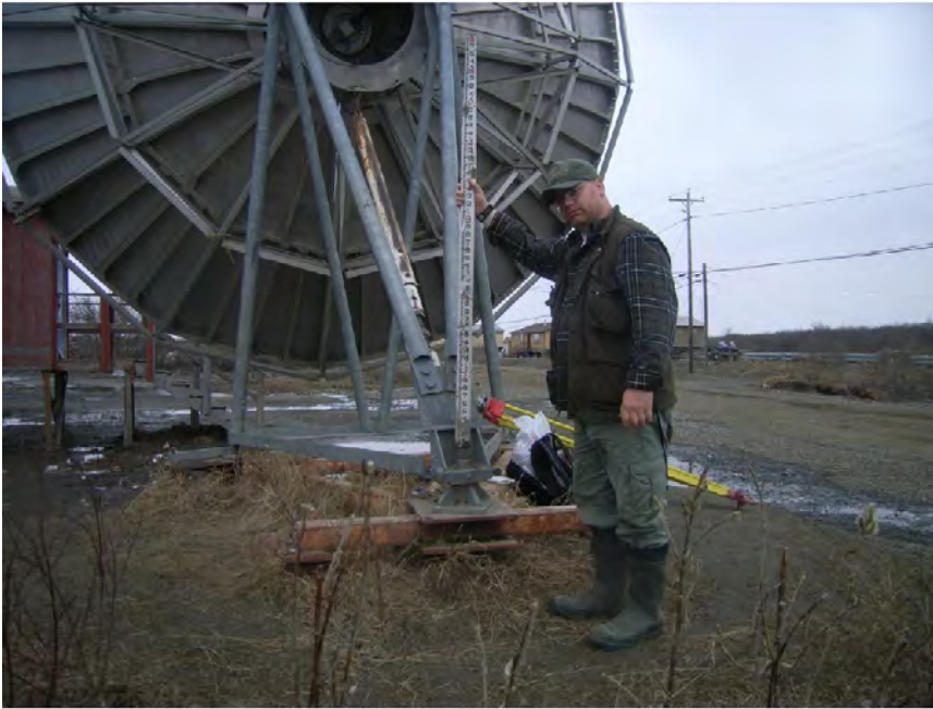
Photo 11: Location of temporary benchmark used for elevation control in Survey Area 2.
