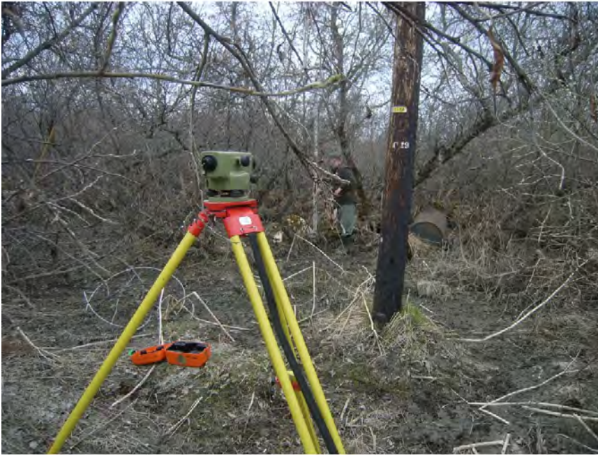
Photo 3: AHW 1 was a silt line found on a moss covered tree.
