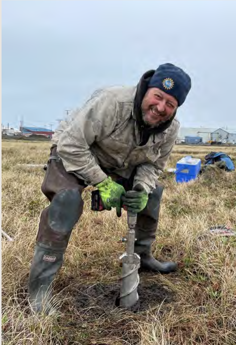
Coring with the SIPRE corer (10 boreholes)
