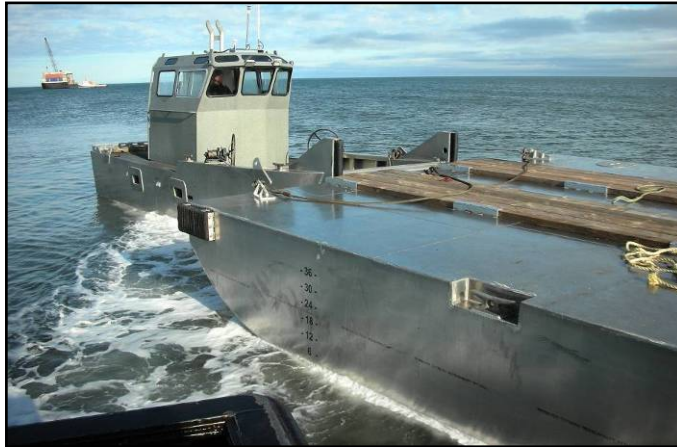
Figure 6.1.3: Shallow draft barge and push boat used to lighter to shore.
