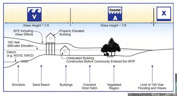
1% Annual Chance Storm (100-Year) Stillwater elevation (tide plus surge) Plus Wave Elevation Plus Wave Run-Up
