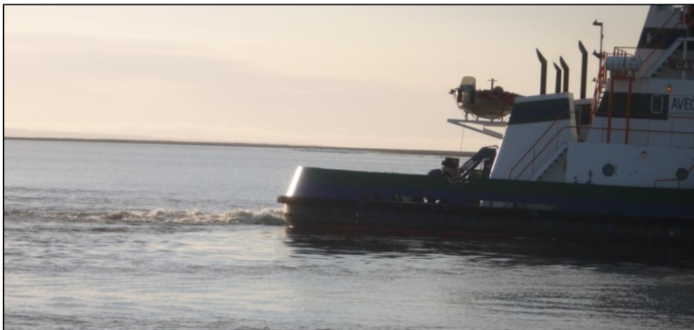
Figure 6. Prop wash from the AVEC barge, while stationary against the bank.
