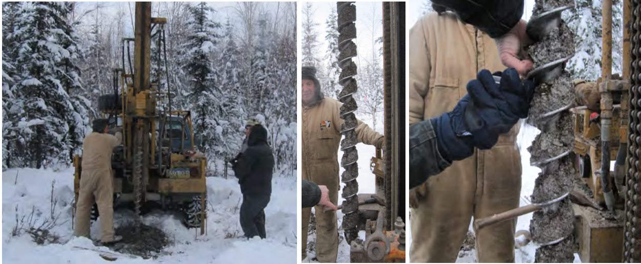
Figure 13. Using an auger to bring up a soil sample. (CCHRC, Inc.)
