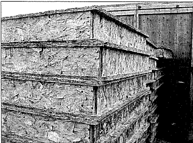
Above: The SIPs uncrated on a prior site visit were left out in the elements and are no longer usable.
