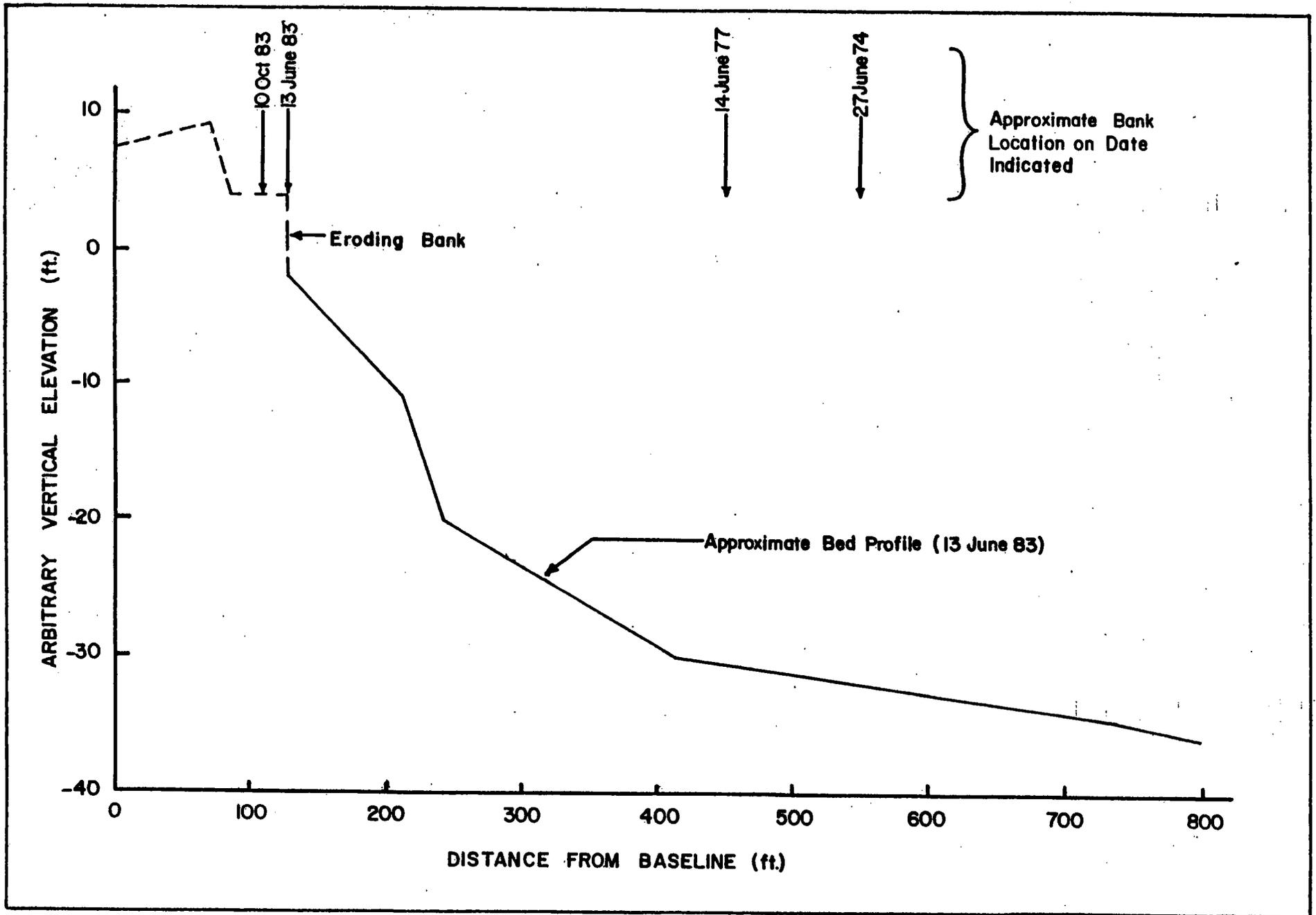
Figure 3. Ninglick River cross-section profile showing depth of bed degradation.
