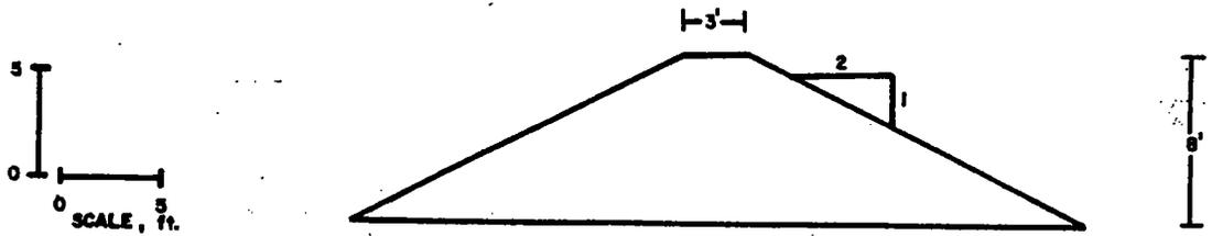
**TYPICAL SPUR DIKE CROSS-SECTION
