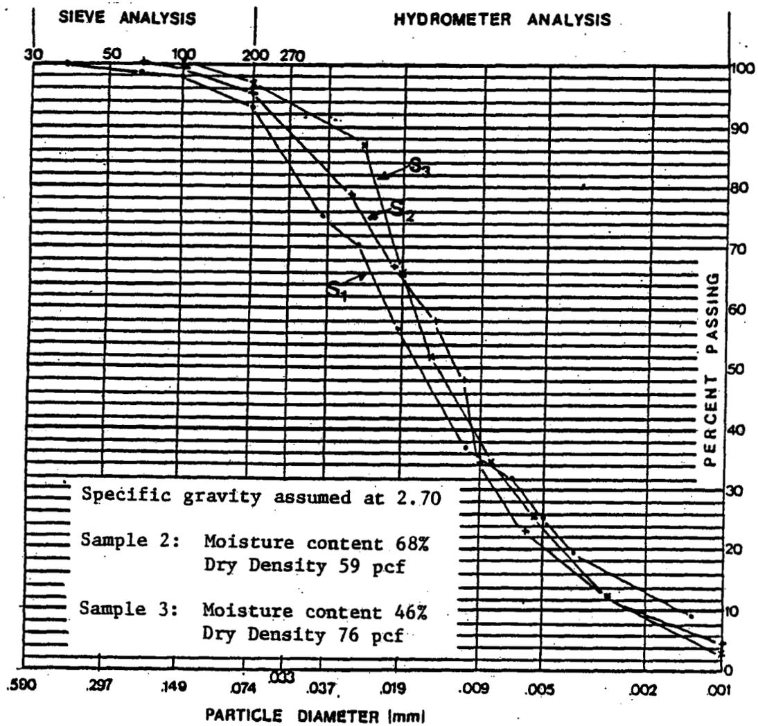
Figure 2. Grain size analysis of bank material samples.
