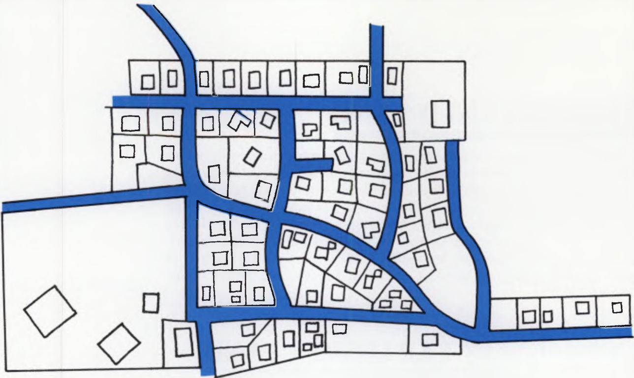
RIGHT-OF-WAY PLAN WITH ADEQUATE ROAD ACCESS
