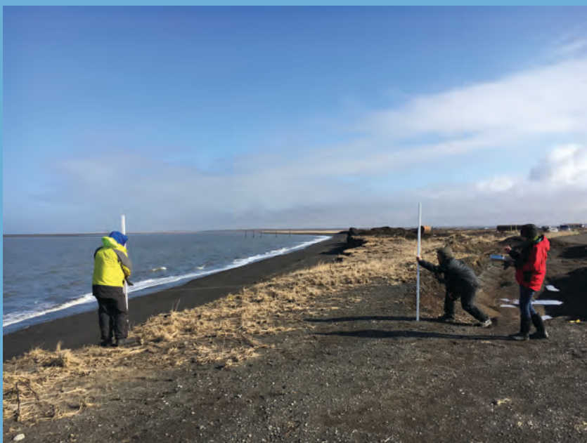
Port Heiden residents measuring erosion and topographic changes using Emery Rods.
