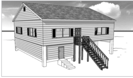
Elevated hanging floor
