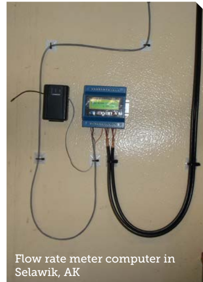
CloudGate router and Ethernet Gateway which act as the hub for the monitoring equipment in Selawik, AK
