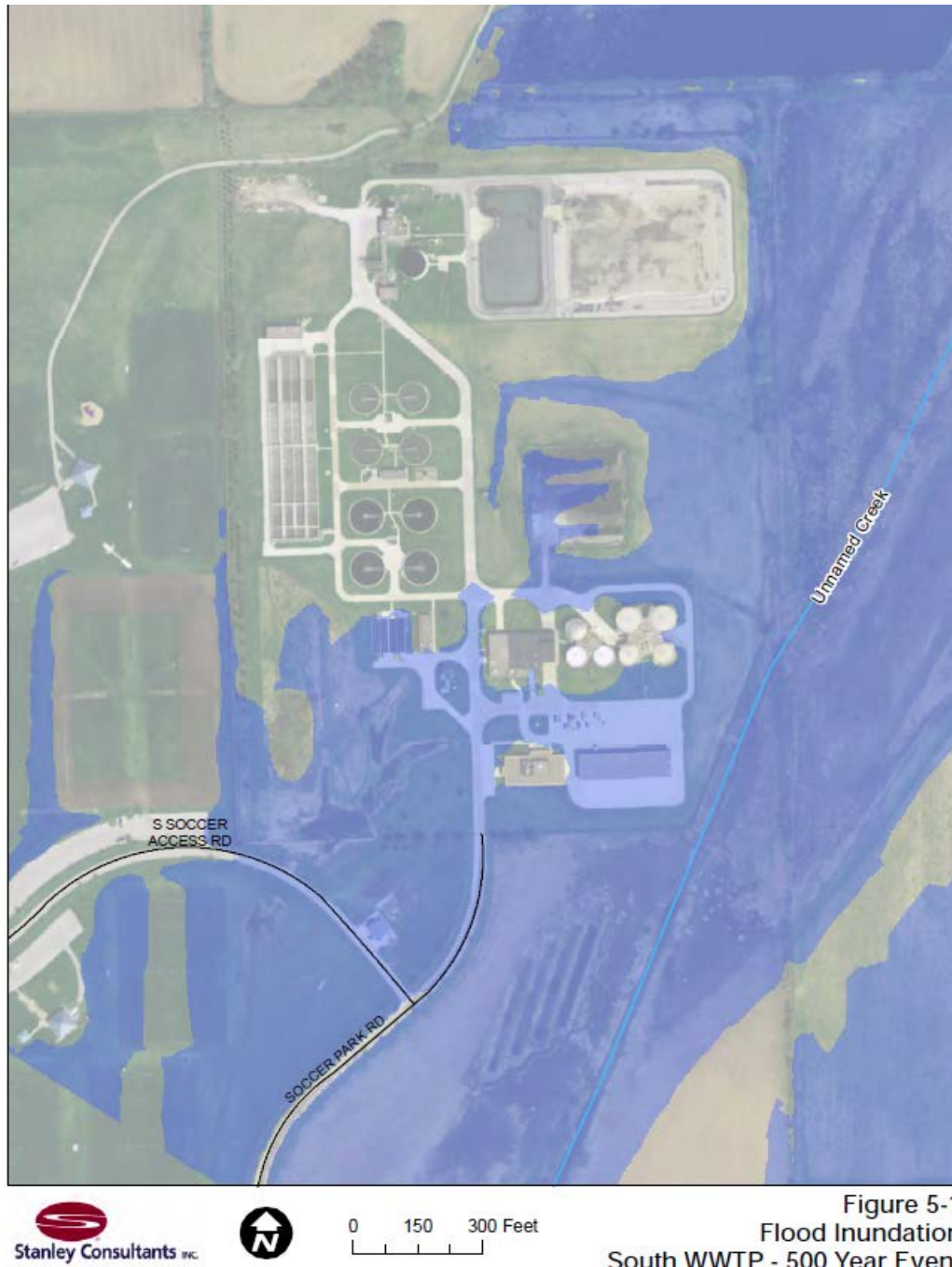
Figure 17. The estimated extent of flooding at the south waste water treatment plant in Iowa City, Iowa, before mitigating sensitive buildings and components, using a 0.2% annual exceedance probability (500-year flood). (Stanley Consultants 2011)
