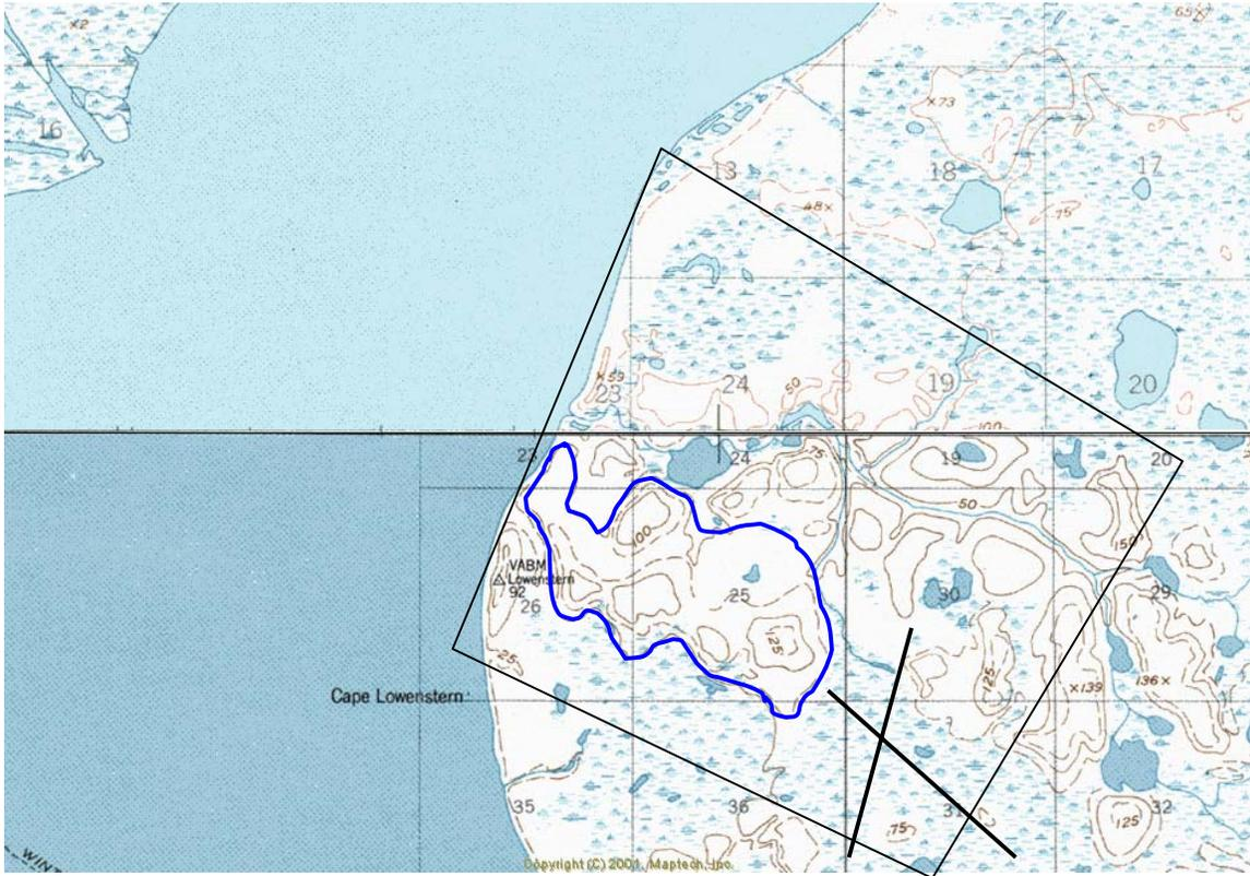
Figure B7 – East Nunatuq location map. Blue outline is the site investigated for the village. Dark black lines are a possible airstrip alignment. Light black lines encompass the original investigation area.
