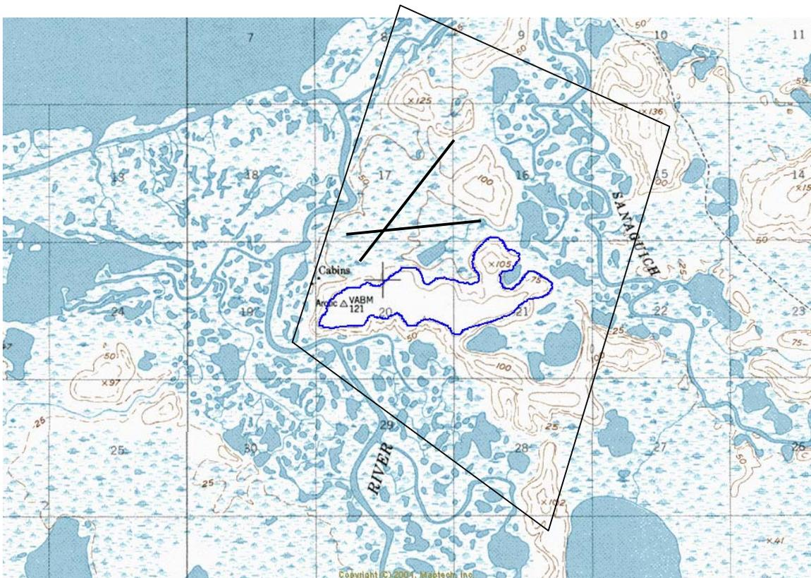
Figure B10 – Arctic location map. Blue outline is the site investigated for the village. Dark black lines are a possible airstrip alignment. Light black lines encompass the original investigation area.
