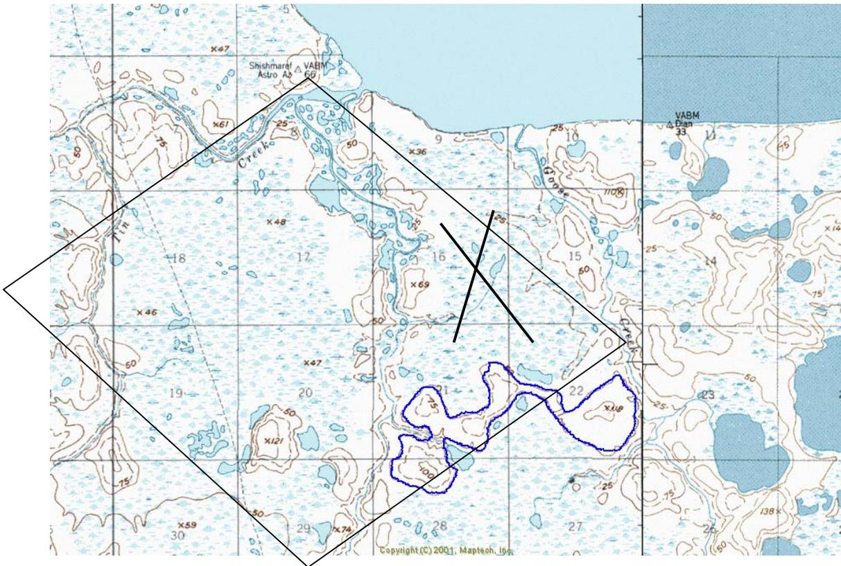
Figure B16 – Tin Creek location map. Blue outline is the site investigated for the village. Dark black lines are a possible airstrip alignment. Light black lines encompass the original investigation area.
