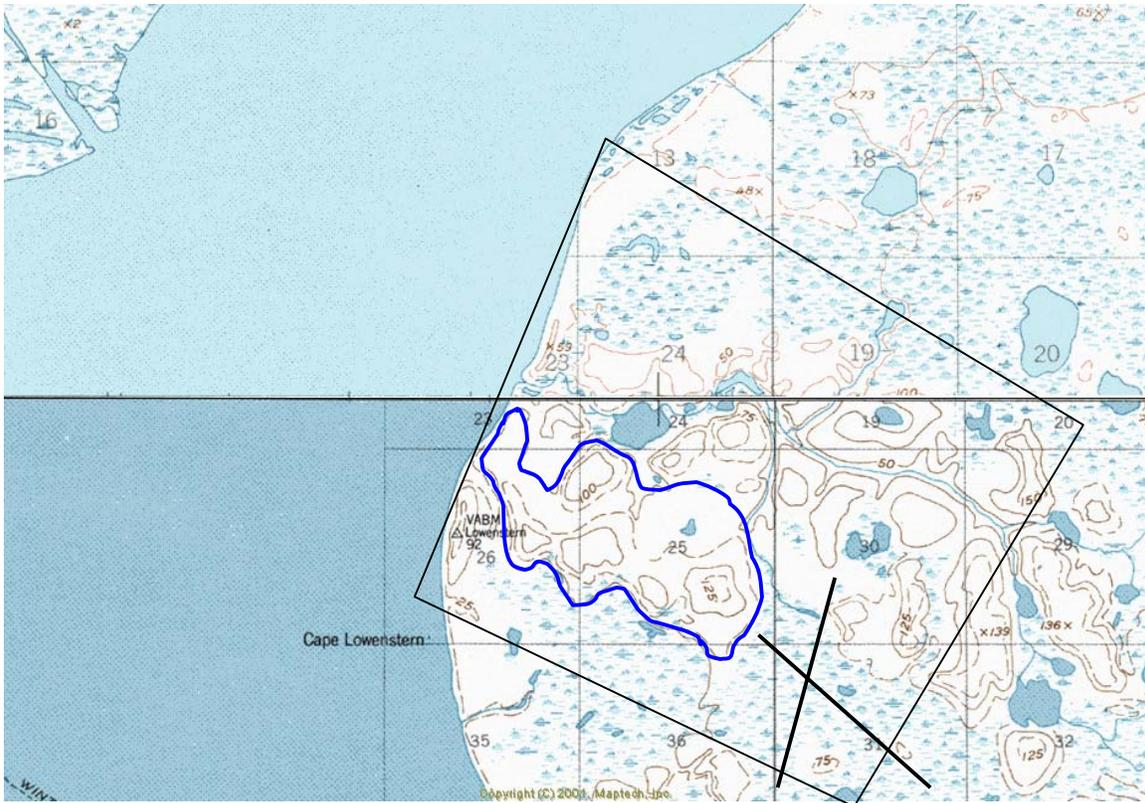
Figure 6 – East Nunatuq location map. Blue outline is the site investigated for the village. Dark black lines are a possible airstrip alignment. Light black lines encompass the original investigation area.
