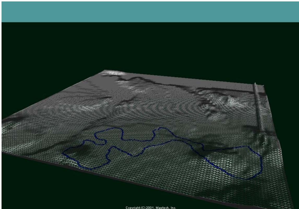
Figure B18 – Tin Creek wire frame model.
