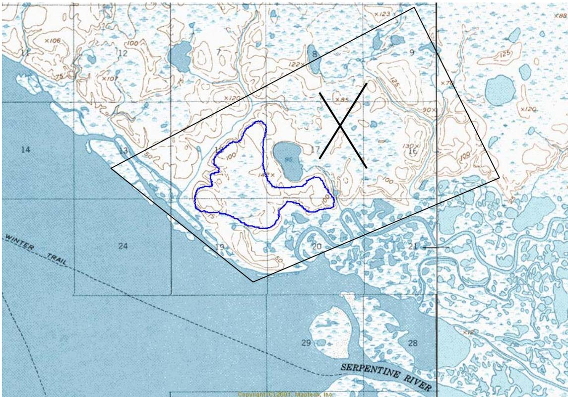
Figure B13 – Igloot location map. Blue outline is the site investigated for the village. Dark black lines are a possible airstrip alignment. Light black lines encompass the original investigation area.
