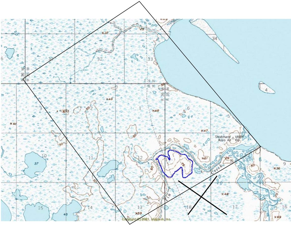
Figure B19 – West Tin Creek Hills location map. Blue outline is the site investigated for the village. Dark black lines are a possible airstrip alignment. Light black lines encompass the original investigation area.
