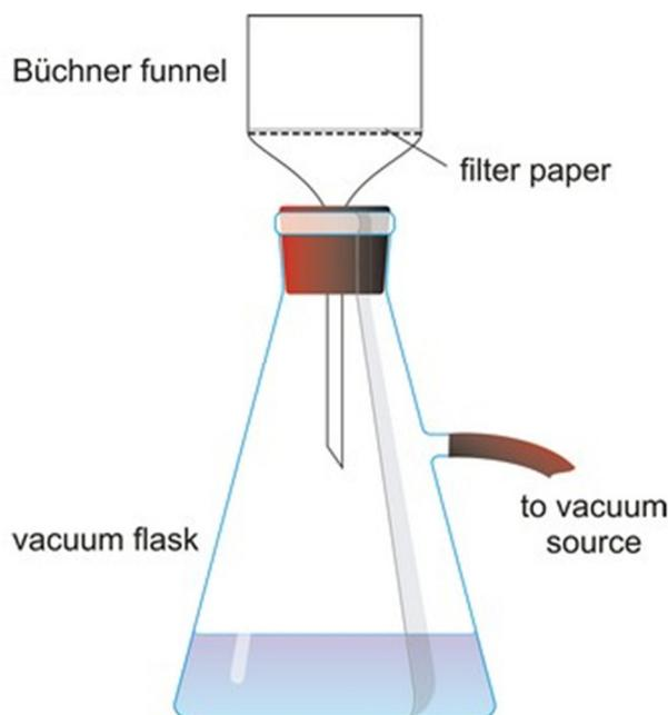
Figure 2: Simple vacuum filtration diagram. Source: <https://glossary.periodni.com/glossary.php?en=vacuum+filtration>
