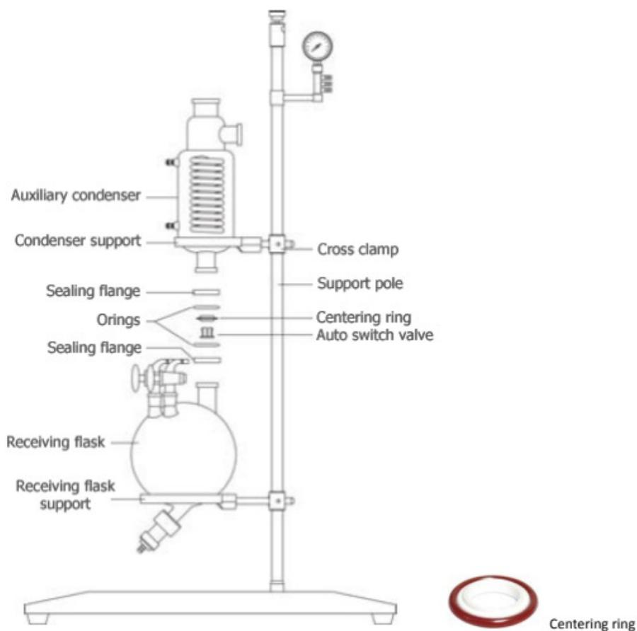
Step 5. Install the vacuum valves according to the illustration below.
