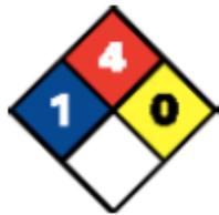
**Figure 1 Example: Butane (See MSDS for exact hazard rating)**
