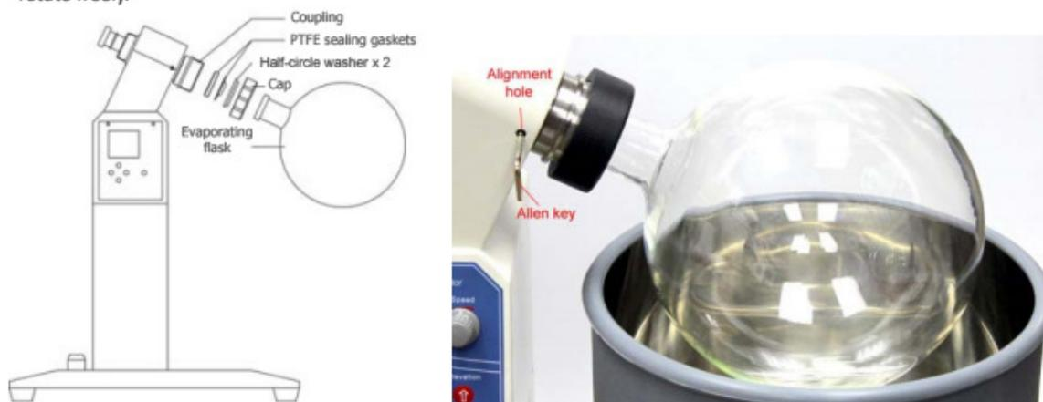
Proper vapor duct PTFE gaskets placement installation
