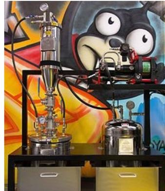
Figure 3: Caresaver Refrigerant Recovery System
